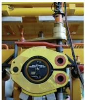
Norbar have developed a torque multiplier specifically for actuating wet pipe connector clamps requiring torques up to 63,000 N.m. The tool is mainly constructed of high strength aluminium to keep the weight within the limits of a standard ROV.
